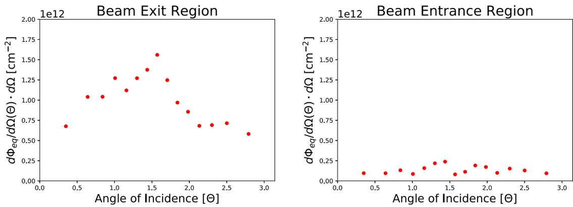
Fig. 8. FLUKA estimates of the angular dependence of the 1 MeV-equivalent neutron fluence through scoring planes in Layer 12 of the BeamCal, for  $10^7$  s of ILC operation. Left: fluence distribution for a scoring plane 24.1 mm beyond the outer edge of the exhaust (larger) circular cutout. Right: fluence distribution for a scoring plane 34.2 mm beyond the outer edge of the incoming (smaller) circular cutout.
