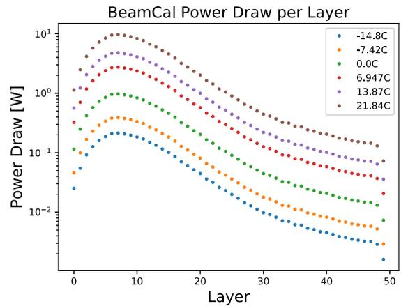
Fig. 14. Expected power draw per layer for operation with a bias voltage of  $V_B = 600$  V after  $10^7$  s of operation in the ILC, for various operating temperatures, under the assumption of charged-particle dominance.
