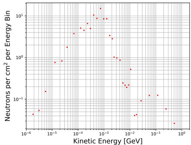
Fig. 7. FLUKA estimate neutron flux, as a function of incident neutron energy, through the sensor scoring plane for Layer 12 of the BeamCal, per ILC beam crossing. The distribution shown is that for a scoring plane centered on the maximum of the electromagnetic component (see Fig. 3). The total estimated per-crossing neutron fluence is given by the sum of the bin contents.
