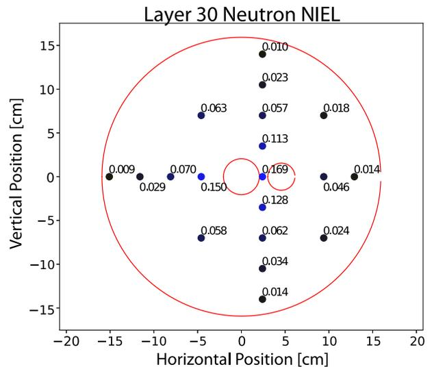
Fig. 11. FLUKA estimate of neutron-induced NIEL for the various scoring planes configured for Layer 30 of the BeamCal. The results are shown per year of ILC running (as defined in the text), and expressed in the T506 dose unit  $\lambda_{T506}$ .
