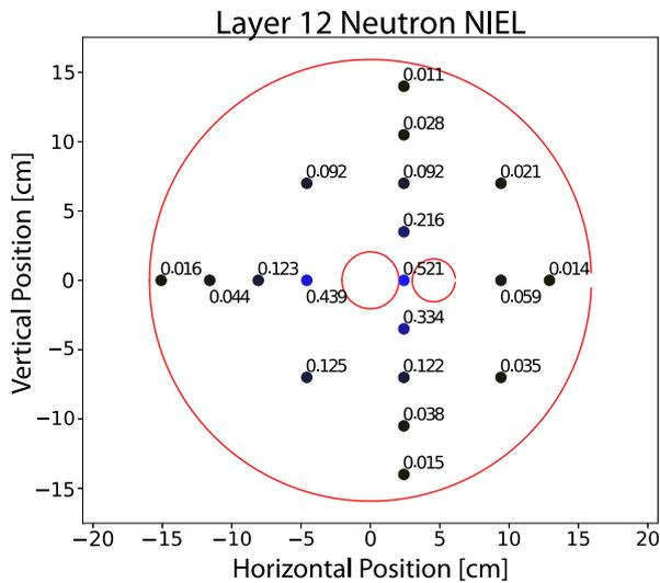
Fig. 10. FLUKA estimate of neutron-induced NIEL for the various scoring planes configured for Layer 12 of the BeamCal. The results are shown per year of ILC running (as defined in the text), and expressed in terms of the T506 dose unit  $\lambda_{T506}$ .
