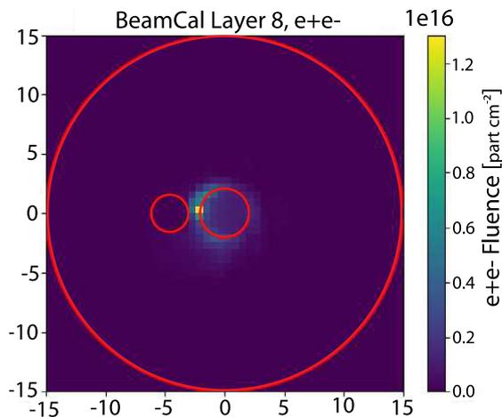
Fig. 3. Estimated electromagnetic (electron and positron) fluence, in cm<sup>-2</sup>, at the maximum of the electromagnetic shower in the BeamCal, per 10<sup>7</sup> s of ILC operation. The estimated maximum occurs in the eighth sensor layer. The outer red circle represents the periphery of the BeamCal, while the larger (smaller) red circles represent the exit (entrance) holes for the ILC beams, also visible in Fig. 1. Distances are in cm.
