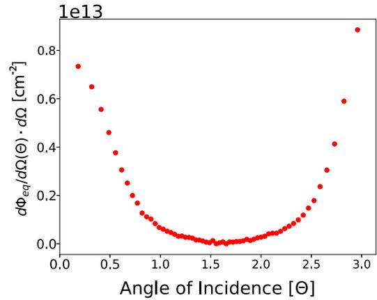
Fig. 6. FLUKA estimate of the angular dependence of the 1 MeV-equivalent neutron fluence through the sensor scoring plane for the full exposure of the T506 experiment.
