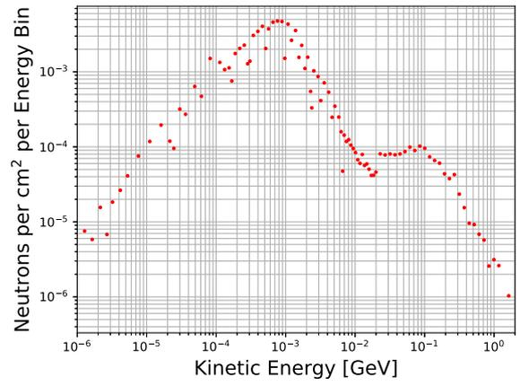
Fig. 5. FLUKA estimate of the neutron fluence per 13.3 GeV primary electron, as a function of incident neutron energy, through the sensor scoring plane for the T506 experiment. The total estimated per-primary neutron fluence is given by the sum of the bin contents.
