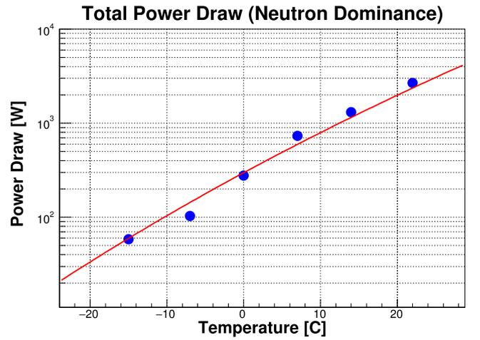
Fig. 13. Expected power draw as a function of temperature for the entire BeamCal after  $10^7$  s of operation at the ILC, for operation with a bias voltage of  $V_B = 600$  V, under the assumption of neutron dominance.
