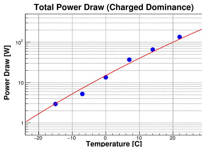
Fig. 15. Expected power draw as a function of temperature for the entire BeamCal after  $10^7$  s of operation at the ILC, for operation with a bias voltage of  $V_B = 600$  V, under the assumption of charged-particle dominance.
