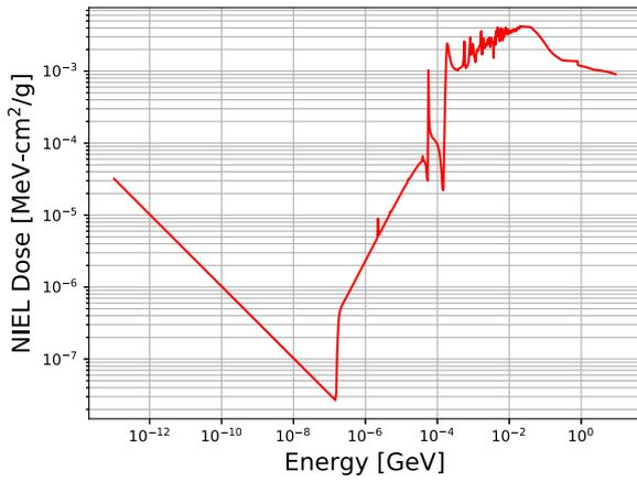
Fig. 4. Energy dependence of neutron-induced NIEL in silicon, in MeV per g/cm<sup>2</sup> of silicon traversed per through-going neutron.
