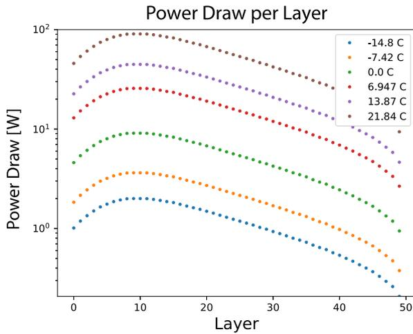
Fig. 12. Expected power draw per layer for operation with a bias voltage of  $V_B = 600$  V after  $10^7$  s of operation in the ILC, for various operating temperatures, under the assumption of neutron dominance.
